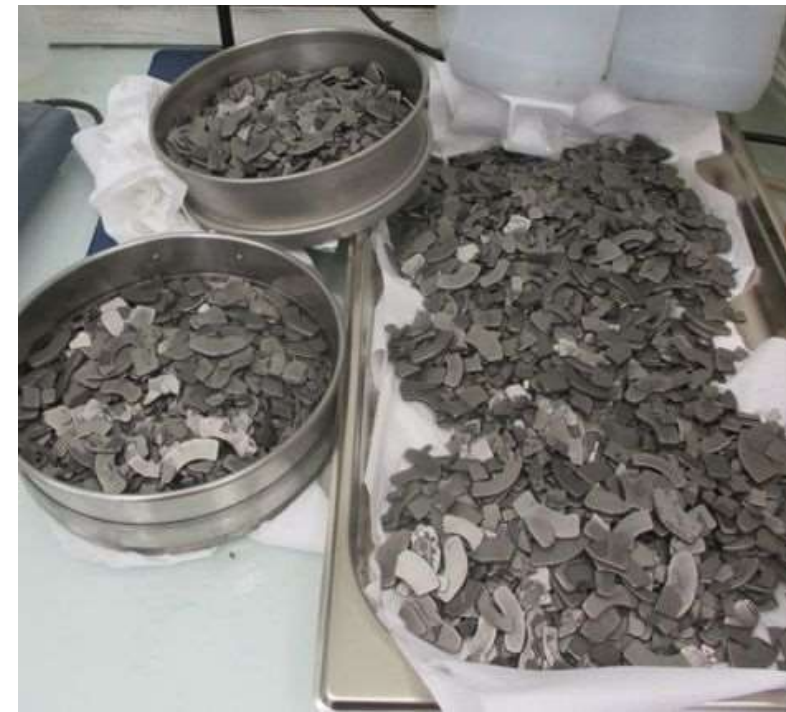
Clean magnets after removal of carbon formed during thermal pyrolysis
