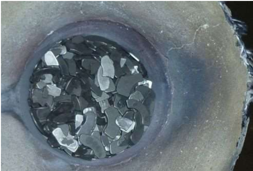
Melting of HDD clean magnets in the strip-casting furnace : SC52
