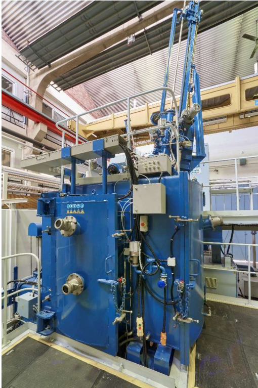
Strip cast equipment installed in CEA – pilot scale
