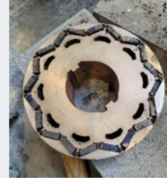
EV and E-scooters rotors with magnets
