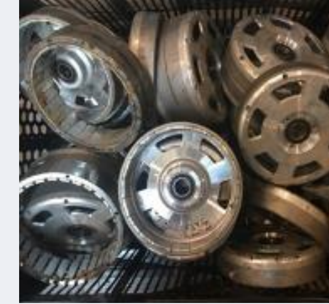
EV and E-scooters rotors with magnets
