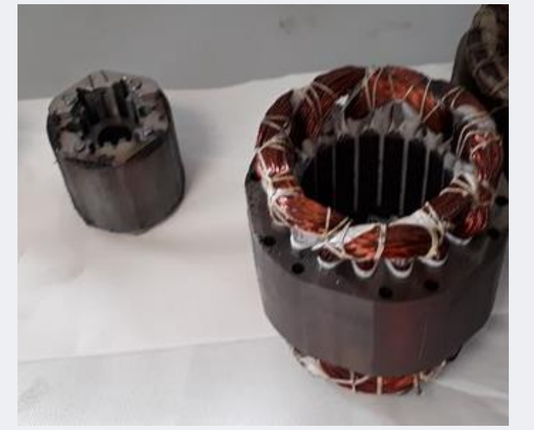
Rotor and stator from air-cooling compressor
