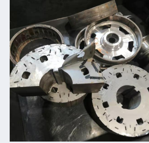
EV and E-scooters rotors with magnets
